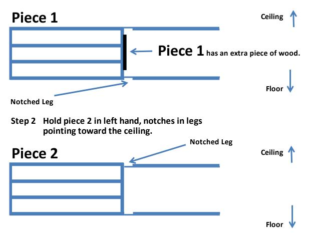
Step 3 Align the notches in piece 1 & 2 and interlock the legs to complete assembly.
